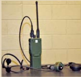
Figure 4 ITT's Rifleman Radio, a lightweight body-worn radio, allows dismounted infantry soldiers and Marines to communicate among themselves and surrounding vehicles, sensors and unmanned vehicles.
