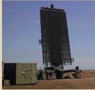
Figure 3 The Three-Dimensional Expeditionary Long-Range Radar (3DELRR) will serve as the ground-based sensor for long-range detection, identification, tracking and reporting of aircraft and missiles for both the Air Force and the Marine Corps.
